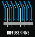
The angular fins largely extend the contact surface of the air and the fins, enabling the air current to transmit in the steadiest way.
