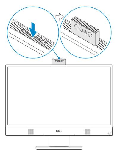
$\bigcirc$  NOTE: Extend the camera while using any camera function so that the camera is not blocked.
