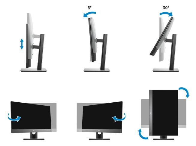
(i) NOTE: When you change the stand orientation from landscape mode to Portrait mode or the other way round, the screen does not automatically change the orientation. Change the screen orientation in the Intel control panel settings.
