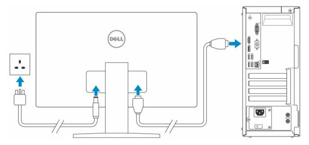
NOTE: If you ordered your computer with a discrete graphics card, the HDMI and the display ports on the back panel of your computer are covered. Connect the display to the discrete graphics card.
