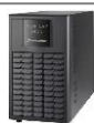
Battery Pack with inside 2x Battery Sets (Each battery set contain 6x 12V/9Ah batteries) Datasheet: Link
