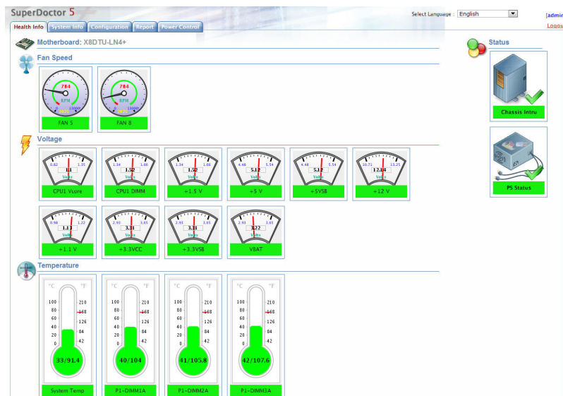
Figure B-2. SuperDoctor 5 Interface Display Screen (Health Information)
