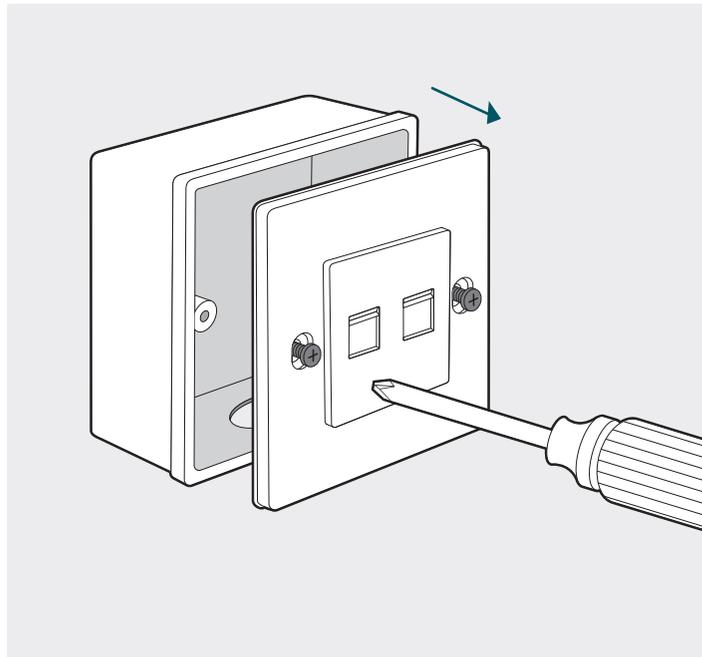
3. Connect the Ethernet cable inside the junction box to an RJ45 plug. Then connect the cable to the UPLINK+PoE port. Position the Ethernet cable to ensure it is not strained.
