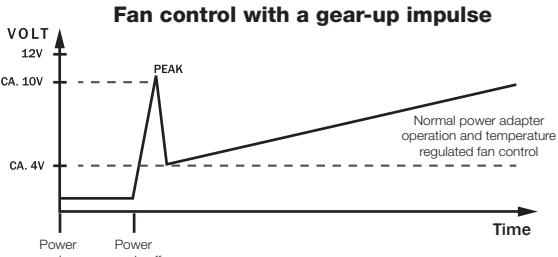
The fan control system generates a start-up signal. This short, high-voltage burst ensures that all the connected fans in the case will start together each time.
