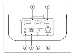
1 HDMI IN 1 / HDMI IN 2 Connect to the HDMI output on a digital device.
