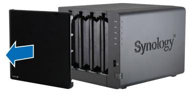
2 Push the latch upward and pull the handle to remove the drive tray.
