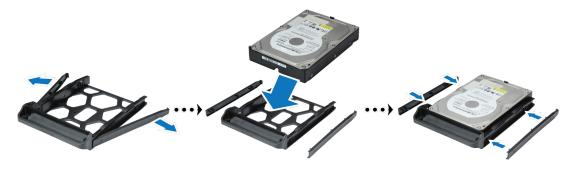
• For 2.5" drives: Remove the fastening panels from the sides of the drive tray and store them in a safe place. Place the drive in the blue area (shown below) of the drive tray. Turn the tray upside down and tighten the screws to secure the drive in place.
