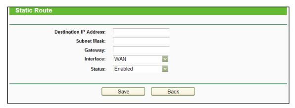
Figure 4-88 Add or Modify a Static Route Entry
