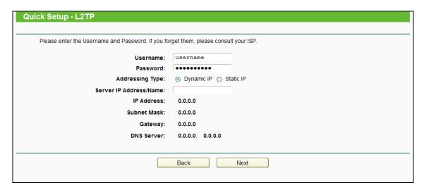
Figure 3-10 Quick Setup - L2TP/Russia L2TP
