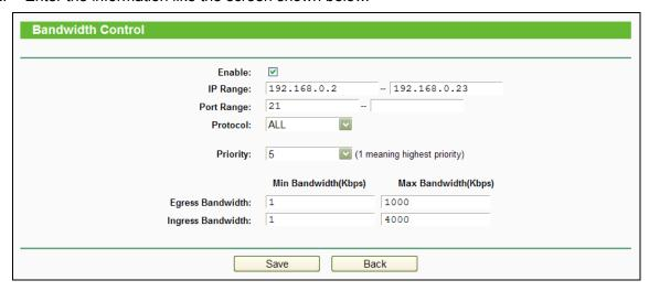
Figure 4-91 Bandwidth Control Rule Settings
