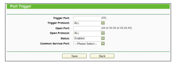
Figure 4-64 Add or Modify a Triggering Entry
