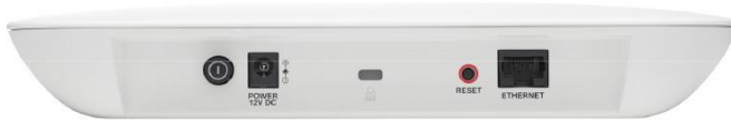
Figure 3. Back Panel of the Cisco WAP371 Wireless-AC/N Dual Radio Access Point with Single Point Setup
