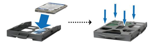
4 Insert the loaded drive tray into the empty hard drive bay.
