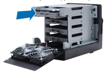
*Important:* Make sure the drive tray is completely inserted. Otherwise, the drive might not function properly.
