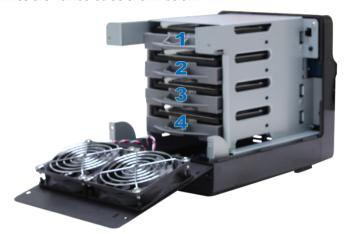
• For 3.5" drives (only): Secure the drive trays with the screws (for securing drive trays) provided, which is not required for 2.5" drive.
