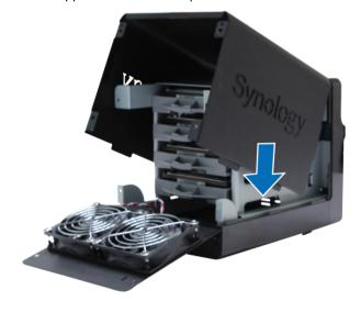
8 Close the back cover. Replace and tighten the 4 screws you removed in step 1.
