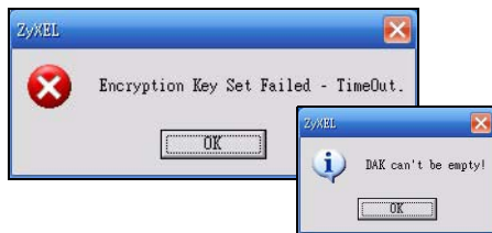
Figure 30 Incorrect DAK or No DAK
