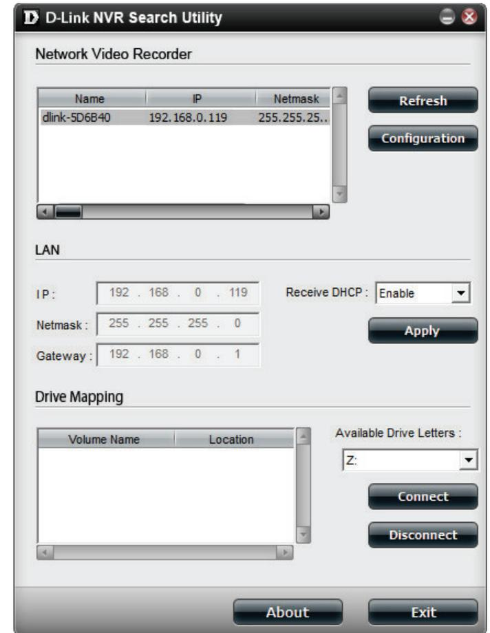
Select the device from the list and click the **Configuration** button. This will launch the computer's default web browser and direct it to the IP address listed for the device. Make sure the browser is not configured to use a proxy server.
