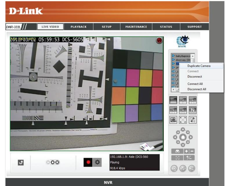
**Duplicate Camera:** Select the duplicate camera function to create multiple views. The duplicated camera will be shown with green indicator. Combine this function with digital PTZ, users are allowed to enlarge different spots and view them in different channels meanwhile record the whole view.
