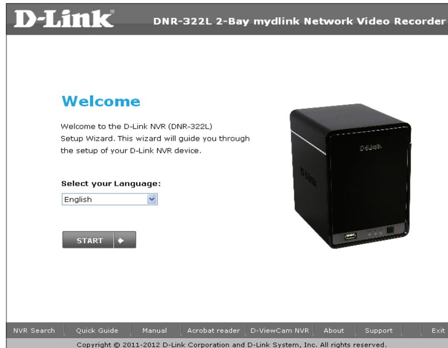
**Note:** The computer used to access the NVR web-based configuration manager must be on the same subnet as the NVR. If your network is using a DHCP server, the NVR will automatically be in the same subnet.
