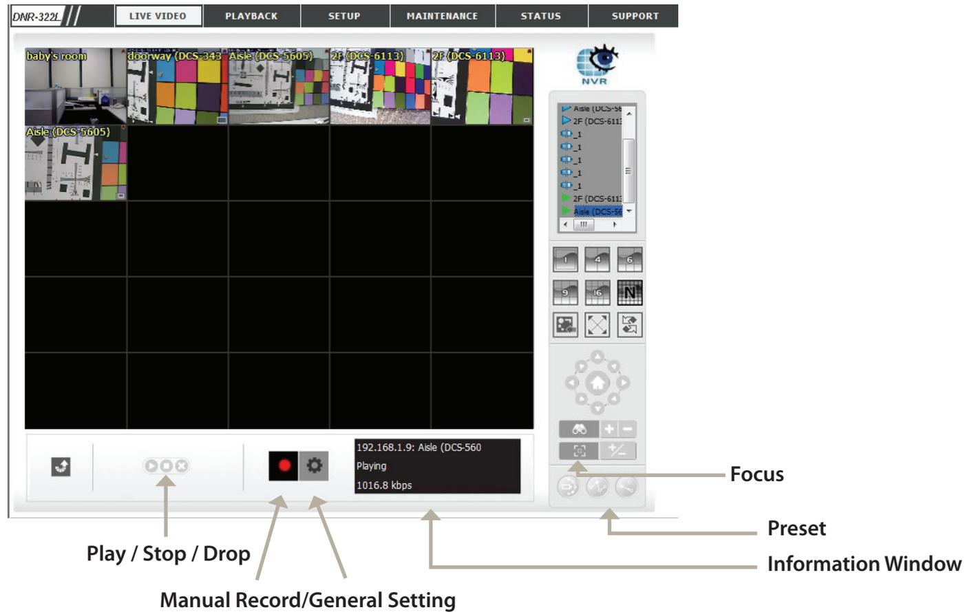
**Preset:** Click the **Set** button to set a preset position for a camera with PTZ support. Users can give the specified position a name and store it in the preset position list. Click the **Go** button to go to the preset position. This is only available with cameras that support the PTZ function.
