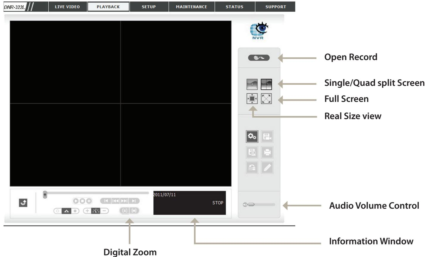
**Single/Quad split Screen:** User may view a single camera or 4 cameras at a time. The DNR-322L only supports 1 camera playback.
