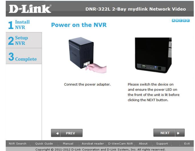
With the power on check that the Power LED is solid. If it is solid, answer **Yes** to the confirmation window otherwise select **No** and wait for the power connection to the NVR. If the connection is good then check that the hard drives are installed correctly and have no other issues. Click **Next** to continue.
