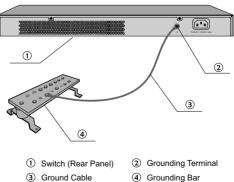
Figure 3-1 Connecting to the Grounding Bar
