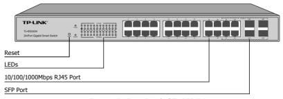
Figure 1-2 Front Panel of TL-SG2424
