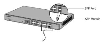
Figure 4-2 Inserting the SFP Module
