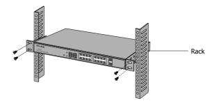
Figure 2-3 Rack Installation
