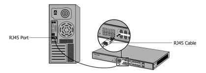
Figure 4-1 Connecting the RJ45 Port
