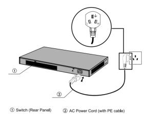
Figure 3-2 Connecting to the Ground
