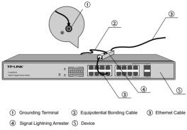
Figure 3-4 Lighting Arrester Connection
