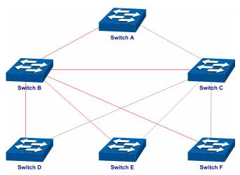
• For Instance 2 (VLAN 102, 104 and 106), the blue paths in the following figure are connected links; the gray paths are the blocked links.
