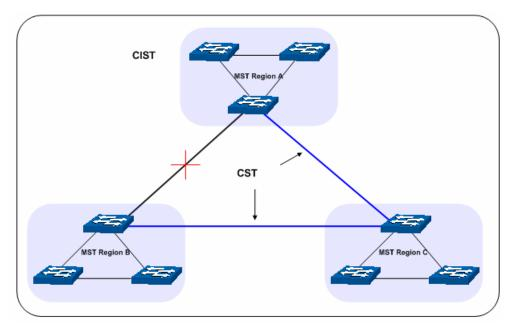
Figure 7-2 Basic MSTP diagram
