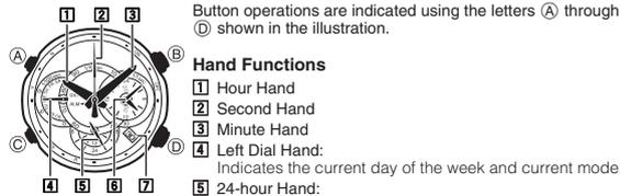
Button operations are indicated using the letters (A) through (D) shown in the illustration.
