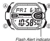
When Flash Alert is turned on, the illumination flashes for the alarms, the Hourly Time Signal, the countdown alarm, and stopwatch (ST1) auto start.
