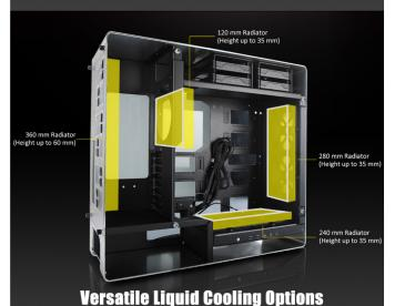
909 has four liquid cooling radiator mounting areas which will allow you to cool specific system components to an even greater degree and provides the best thermal performance.
